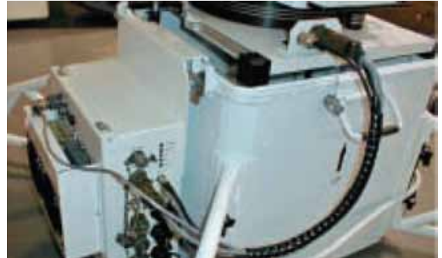
Typical Outdoor Unit with SCPC Modem
