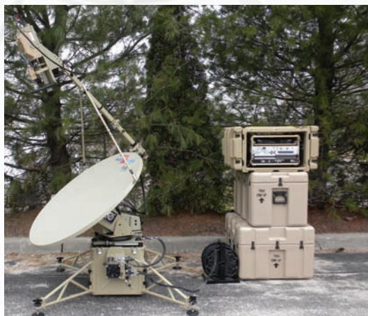
Band specific feed cartridges with Integrated RF Electronics enable quick and simple frequency conversion in the field.
